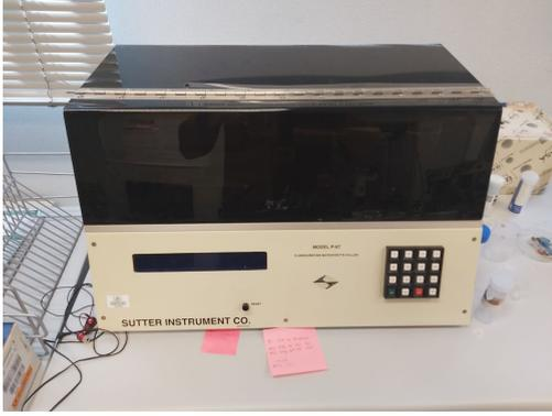
**Figure 8:** Puller used to pull sharped micro-electrodes for the intracellular recordings.
