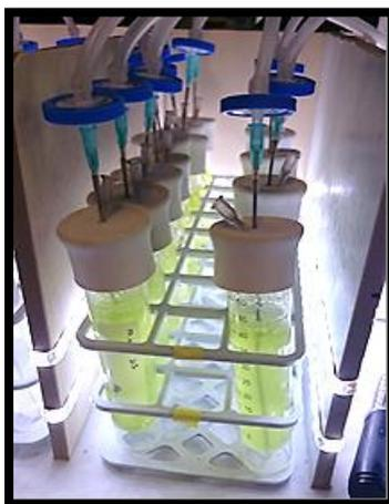
*Figure 3.1. Configuration of the algae culture vessel*
